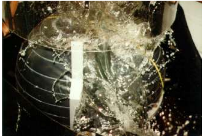
Figure 2: Puncture of the PVC-P membrane at maximum elongation
